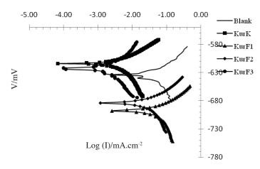
FIGURE 1. Polarization curves for carbon steel in 1% NaCl solutions with various fractions of curcuminoids
